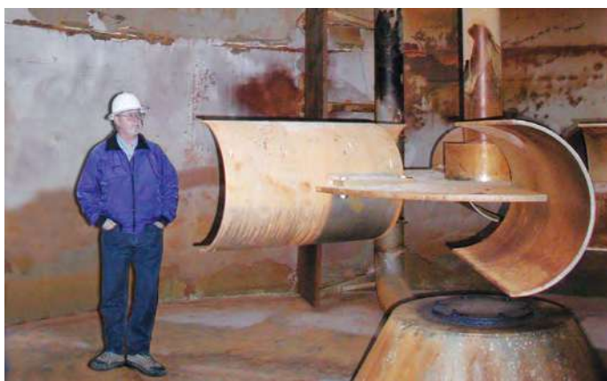
Chemineer agitators can be equipped with a large range of impeller styles and sizes
