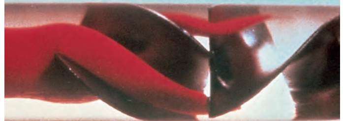
The Kenics heat exchanger directs the flow of material radially toward the pipe walls and back to the element for the most efficient thermal transfer
