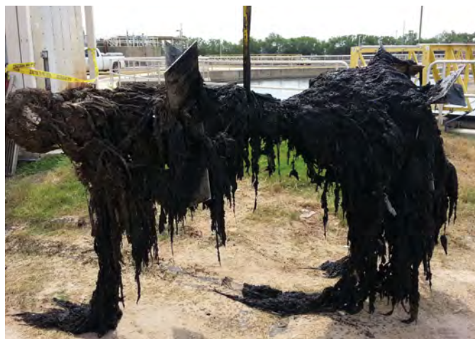
Fibrous build up of a competitive ragless impeller
